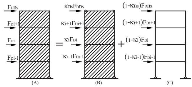
Fig. 12. Decompositions of lateral forces and SPSW system
