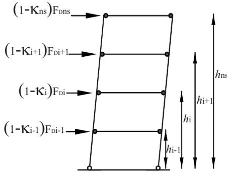
Fig. 13. Plastic mechanism of boundary frame
