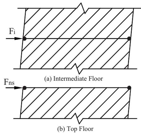
**Fig. 9.** Segments of a uniformly yielded multistory SPSW
