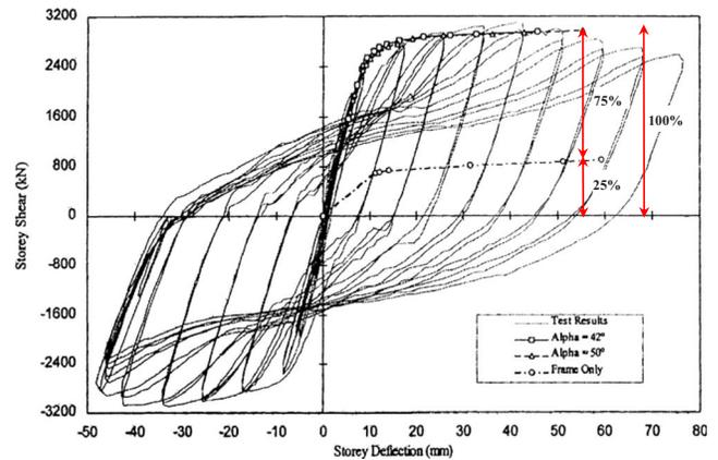
Fig. 3. Test results of a multistory SPSW [adapted from Driver et al. (1997)]
