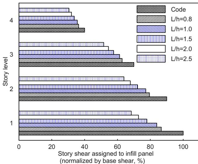
Fig. 11. Modified design forces of an example four-story SPSW
