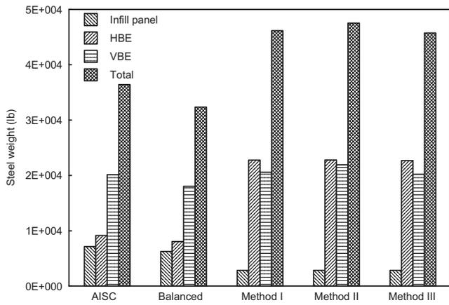
Fig. 15. Comparison of steel weight
