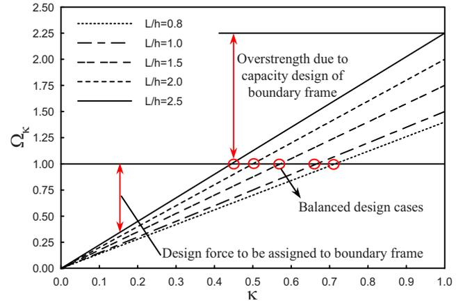
Fig. 5. Relationship between  $\Omega_{\kappa}$  and  $\kappa$  (assuming  $\alpha=45^\circ$  and  $\eta=1.0$ )
