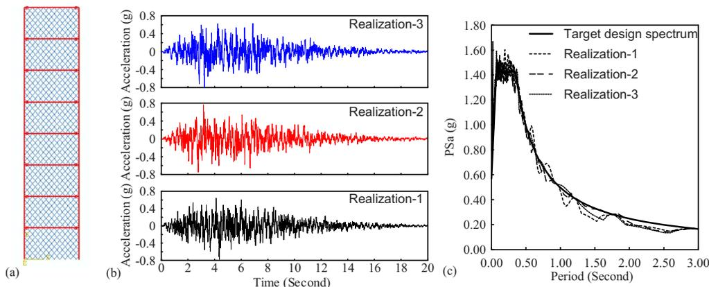
Fig. 16. Dual strip model and ground motion information: (a) dual strip model; (b) ground motion histories; and (c) pseudoacceleration spectra
