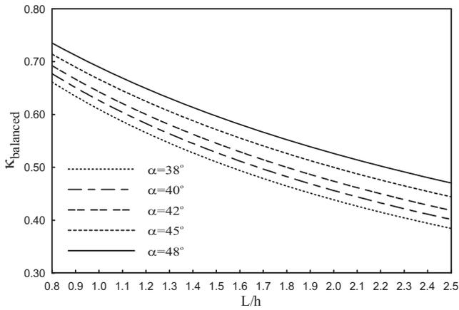
**Fig. 7.** Relationship between aspect ratio ( $L/h$ ) and  $\kappa_{\text{balanced}}$  (assuming  $\eta=1.0$ )
