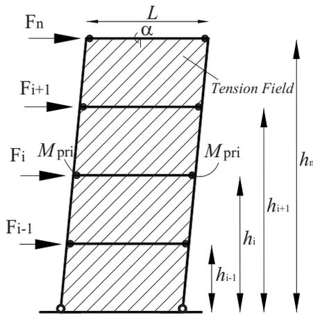
Fig. 1. Desired SPSW plastic mechanism
