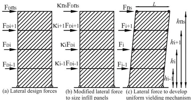
**Fig. 8.** Schematic of a typical multistory SPSW
